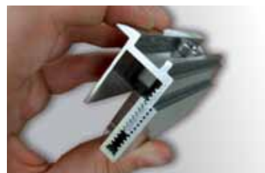
④ Adjust the height-adjustable Rapid 2+ end clamp, snap it in and screw it, respectively use fixed end clamps.
