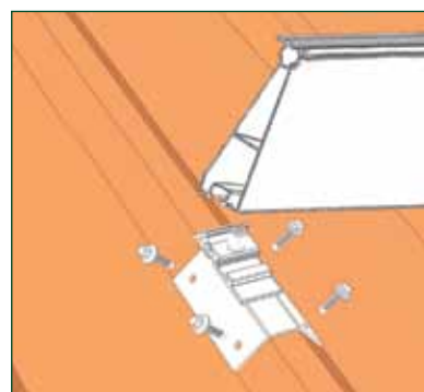
❶ Mounting of the Fix2000ClickTop connector.
